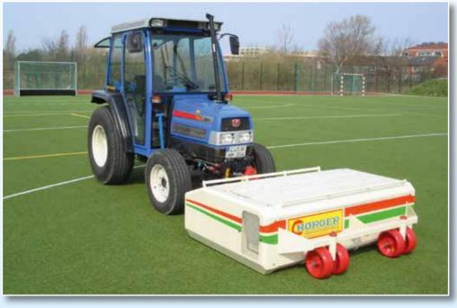
the infill. The bent turf fibres must be reset upright and the infill material installed back into the turf fibres to stabilise them. The surface must appear even to the eye after treatment.
