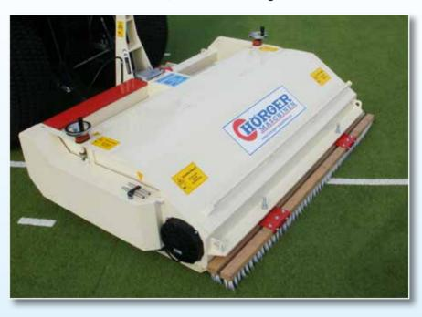
Working width 1.50 m Rear PTO operation 540 r / min
