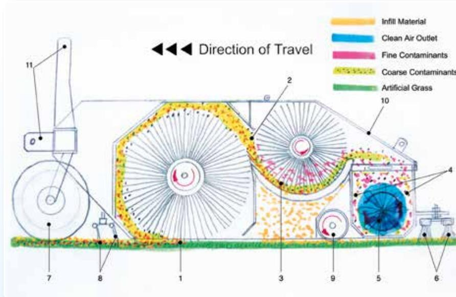
1. The contaminated infill material such as sand, rubber granules or granular sand mixture is taken from the grass surface by a rotating brush.
