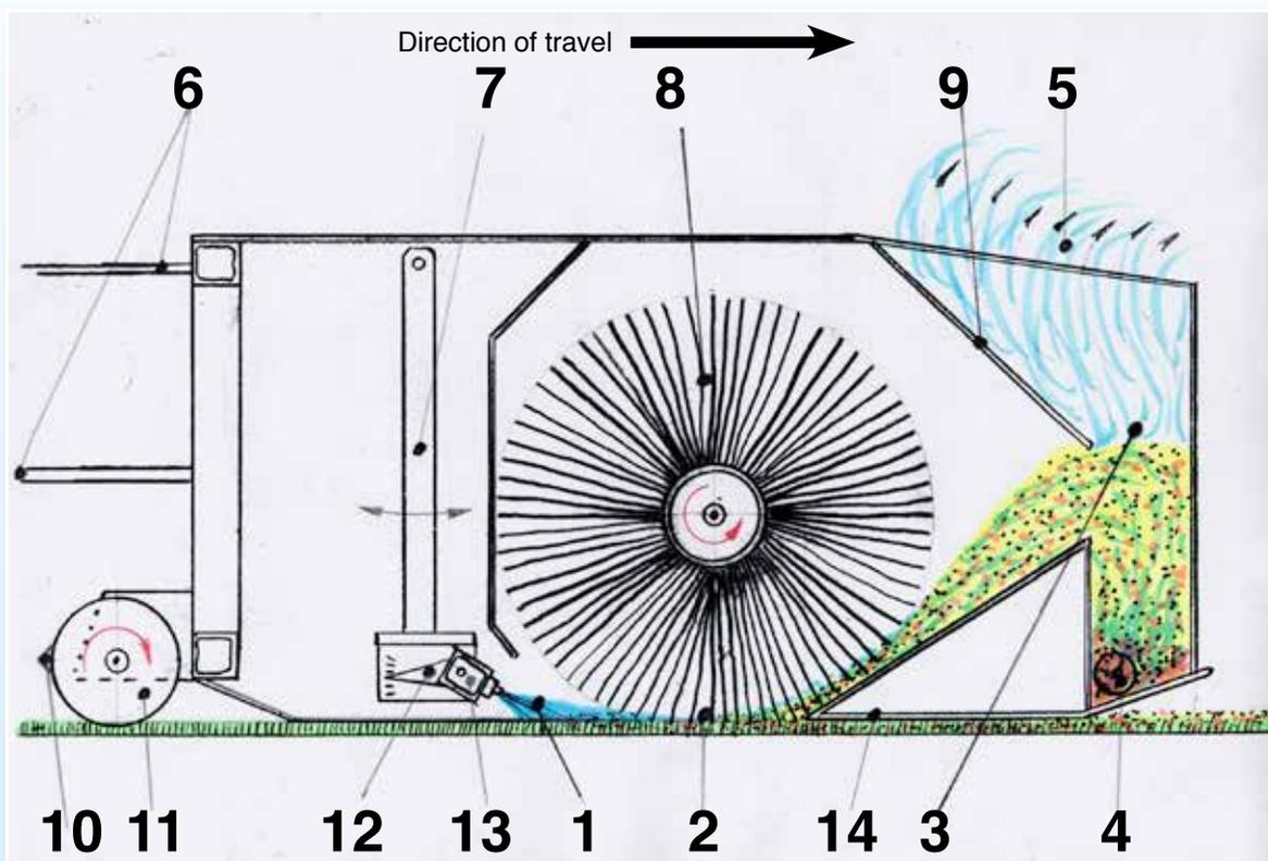
1. From the washing bar, which is tilt-adjustable, cleaning water is jetteted onto the surface to be cleaned under high pressure; in this process, the dirt is flushed out and fed into the rotating brush (8).
