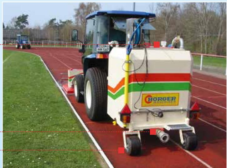
**Demands on the carrier vehicle: Front and rear lift equipment with drive shaft, max. outside width up to 1.45 metres, suitable**
