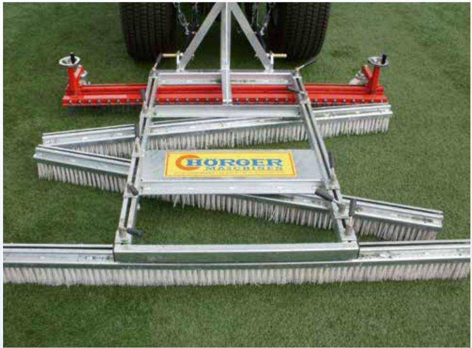
1. Spring steel rake to loosen areas of compacted infill.
